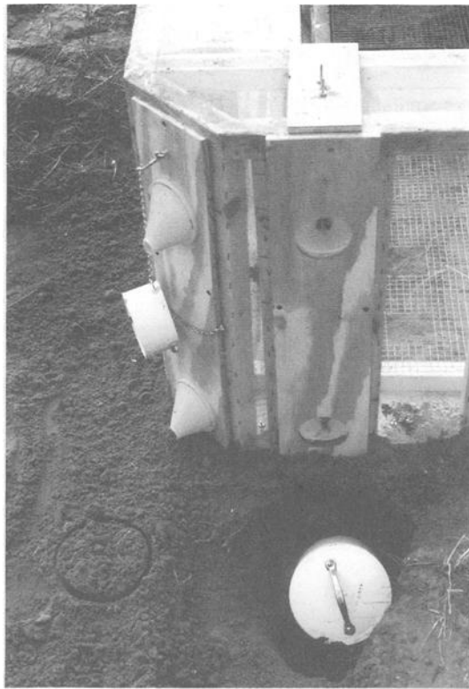
FIG. 12—Final field placement should insure that the bottom rims of all ground level funnels are flush with the surrounding soil. No gap should exist between the screen floor and the undisturbed plot inside. The perforations in the screen floor (see square holes) allow the investigator to collect soil samples from the trap interior.
