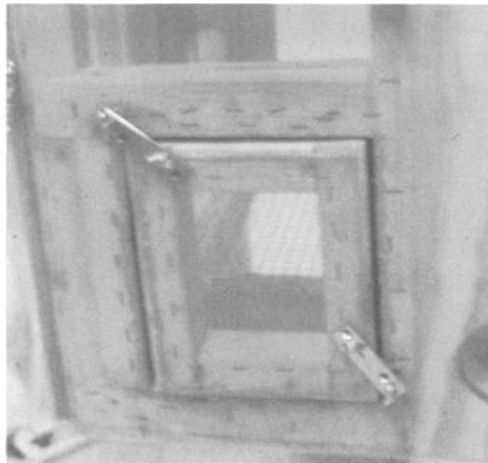
FIG. 9—Close-up of one of the two side doors (15 by 15 cm) for collecting soil and tissue samples and retrieving meteorological instruments (compare with Fig. 1). Each door is fastened to the trap wall with two removable wing nuts.
