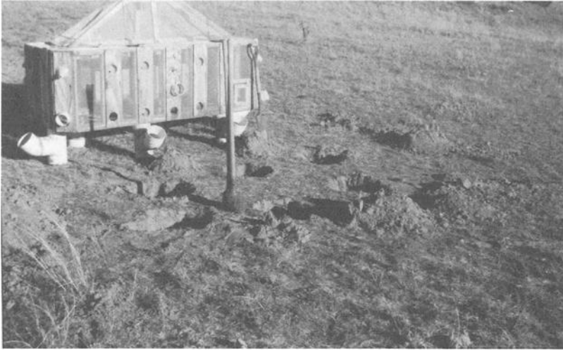
FIG. 11—Field plot shown after excavation of the six conduit holes. These holes guide excavation of the 25-cm-wide by 3-cm-deep trench. The inside rectangular plot (bounded by the trench) is left undisturbed for cadaver placement.
