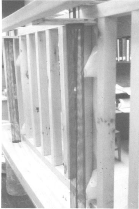
FIG. 5—Two of the six funnel-baffle-pitfall units for capturing immigrating insects (the two vertical screen cylinders shown in the right foreground and left background) (compare with Fig. 4). This photo was taken during an early phase of trap construction.
